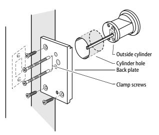
Figure 4 — Installing the outside cylinder
