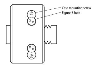
Figure 2 — Removing the case mounting screws
