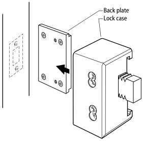
Figure 6 — Sliding the lock case onto the back plate
