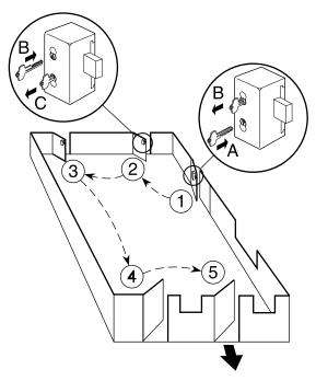
Figure 1 — Using the 23F to enforce unlocking doors in a sequence
