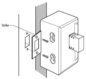
Figure 7 — Installing the strike
