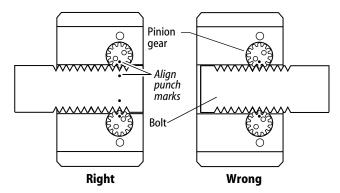
Figure 5 — Re-meshing the bolt and pinion gears
