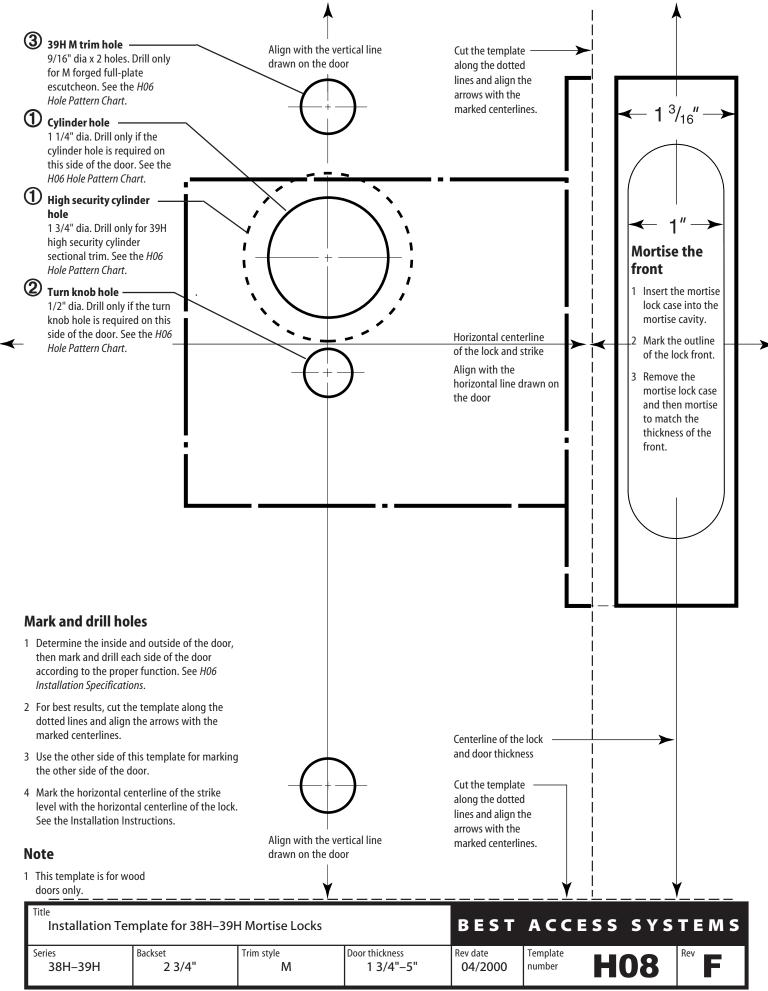
Note: To ensure accurate door preparation, use only factory-printed or laser-printed templates. Do not use copies or facsimilies.
