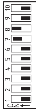
Figure 16 Setting DIP switch 7 to ON to enable door position sensing. (DIP switch 8 is set to ON as a factory default.)
