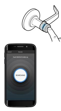
• Touch the **Switch Core** to wake it up. The blue light in the Switch Core will light up.
