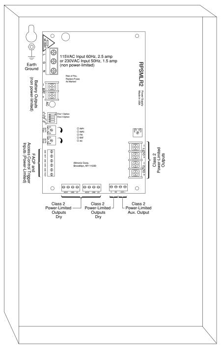
Keep power-limited wiring separate from non power-limited. Use minimum 0.25" spacing.
