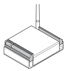
Using the Wireless Access Controller (Figure 12), controllers or other I/O devices can be added to an overall wireless solution without the high cost of installing conduit such as RS485 or CAT5 to the controller. Position the controller at the door or where suitable above the ceiling tile.
