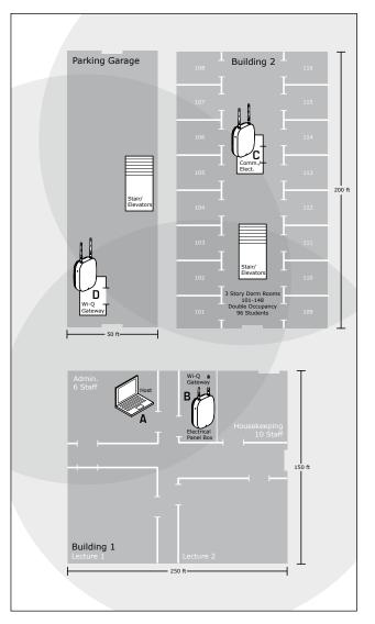
When moving on to configure the Access Control Software, it is essential to have a list identifying each controller and Gateway recognized by the system. We recommend creating a temporary label for each device that includes the MAC address, device name, location, capacity, and type of antenna so that installers on the site will have a reference for installing the correct device in a location.
