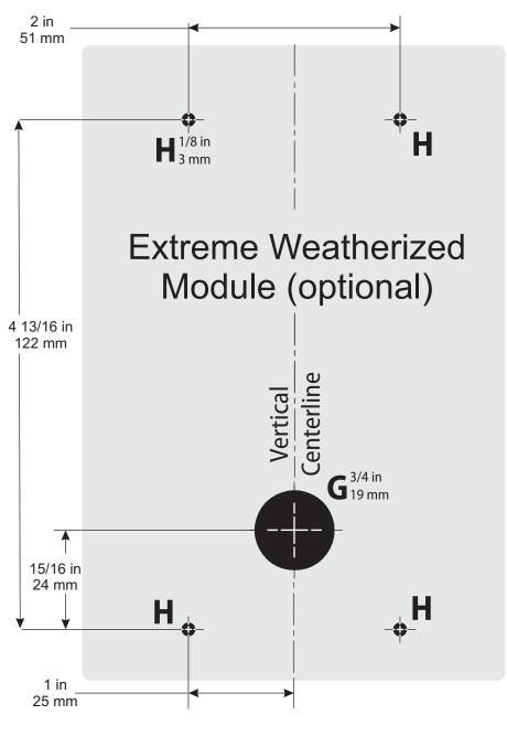
Align the Extreme Weatherized module template as close to the exit device chassis as practical.
