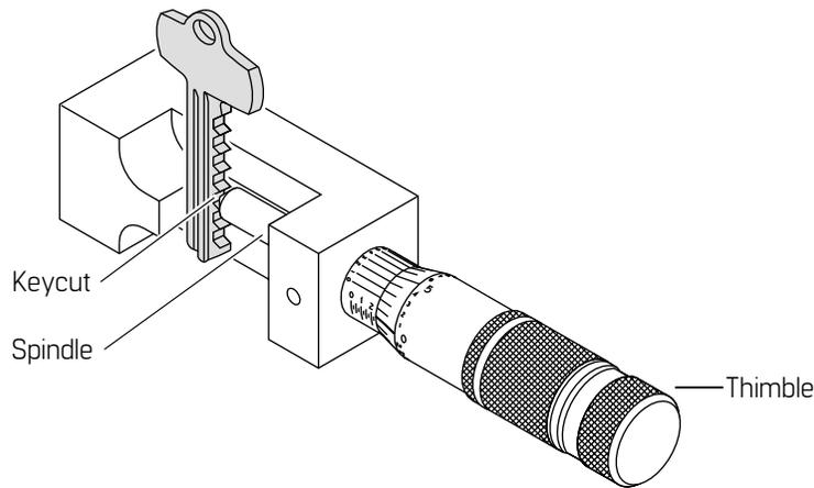
**Figure 3.15** Inserting a key into the key gauge
