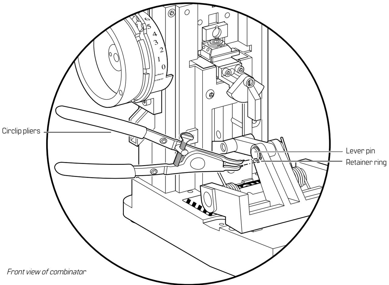
**Figure 3.12** Removing the operating lever
