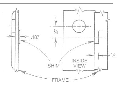
3. FOR FRAMES LESS THAN 3/16" THICK, ATTACH A SHIM (NOT FURNISHED) TO THE INSIDE OF THE FRAME BY BRAZING, SCREWS OR ANY OTHER SUITABLE METHOD SO THAT THE LATCH AREA OF THE FRAME IS .187" THICK. IT SHOULD BE MOUNTED FLUSH WITH THE FRAME AND ON THE CENTER LINE OF THE LATCH TO USE THE A-7175 SERIES.
