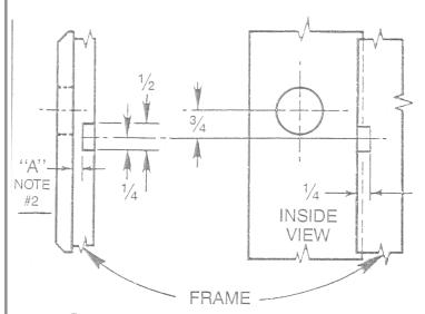
2. FOR FRAMES THICKER THAN 3/16", CUT A 1/2" x 1/4" SLOT IN THE FRAME, 3/4" BELOW THE CENTER LINE OF THE HOLE IN THE DOOR. CUT THE SLOT SO THAT DIMENSION "A" OF THE FRAME REMAINS.
