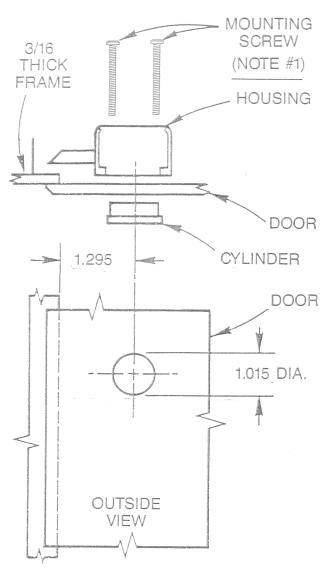
DRILL A 1.015" DIAMETER HOLE IN THE DOOR, 1.295" FROM THE EDGE OF THE FRAME. INSERT THE CYLINDER INTO THE HOLE FROM THE OUTSIDE. TIGHTEN THE HOUSING SECURELY TO THE CYLINDER WITH THE TWO MOUNTING SCREWS PROVIDED. KEEP THE LATCH PERPENDICULAR TO THE EDGE OF THE DOOR. CHECK FOR CORRECT OPERATION. IF THE FRAME IS NOT 3/16" THICK, SEE STEPS 2 AND 3.
