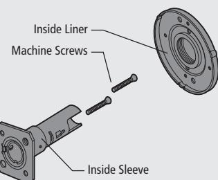
**For 7KC Single Dummy Trim:** Fasten the liner and sleeve assembly onto the door with the screws provided.
