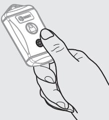
To test FOB functionality, press and hold test button up to 2 seconds. Test button flashes red, then green, indicating successful connection.
