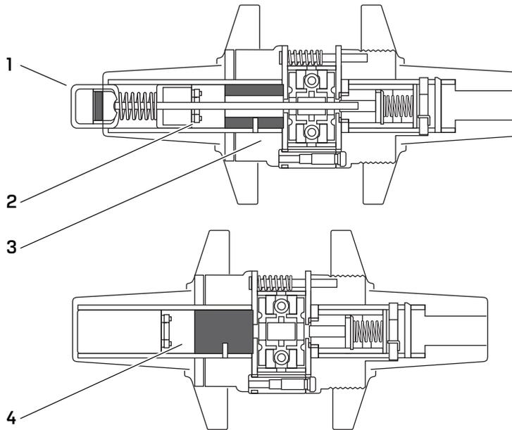
**Figure 2.37** Cross-section of 9K locks showing lead-lined parts
