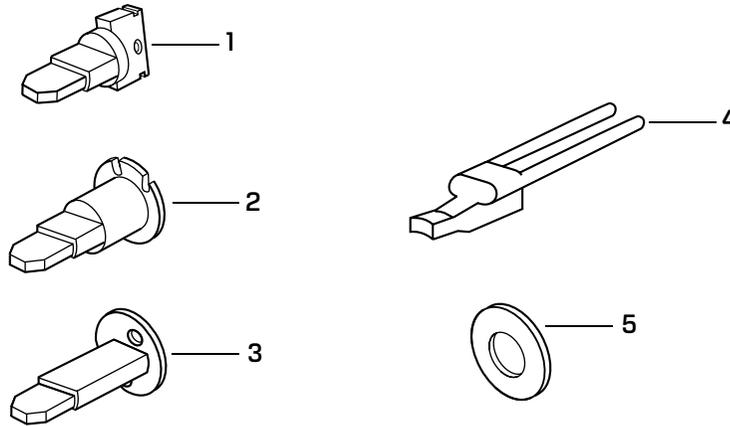
Figure 2.42 Lever components for use with non-interchangeable cores
