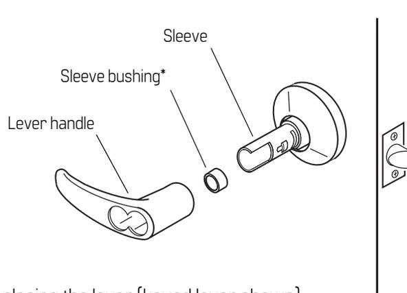
**Figure 3.4** Replacing the lever (keyed lever shown)
