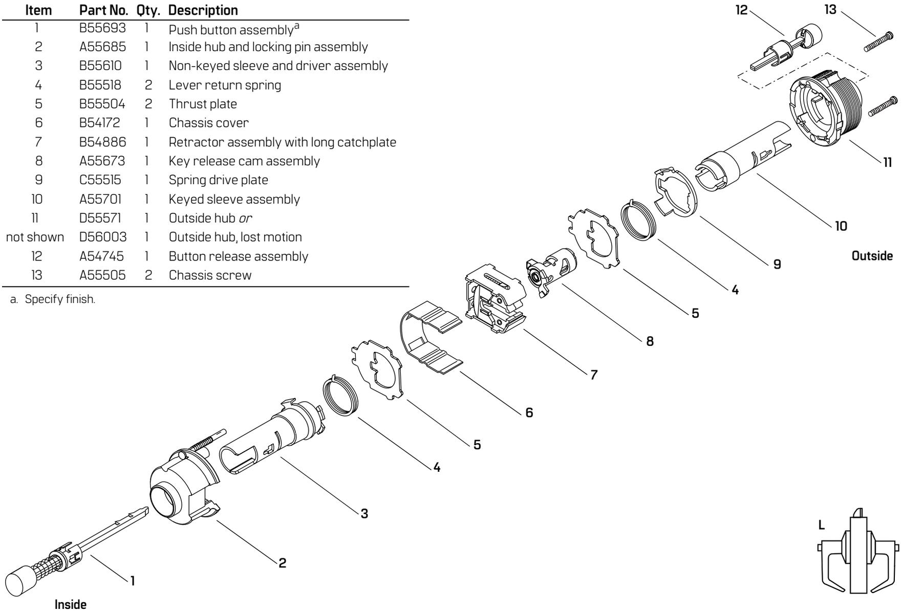
Figure 2.8 L function exploded diagram
