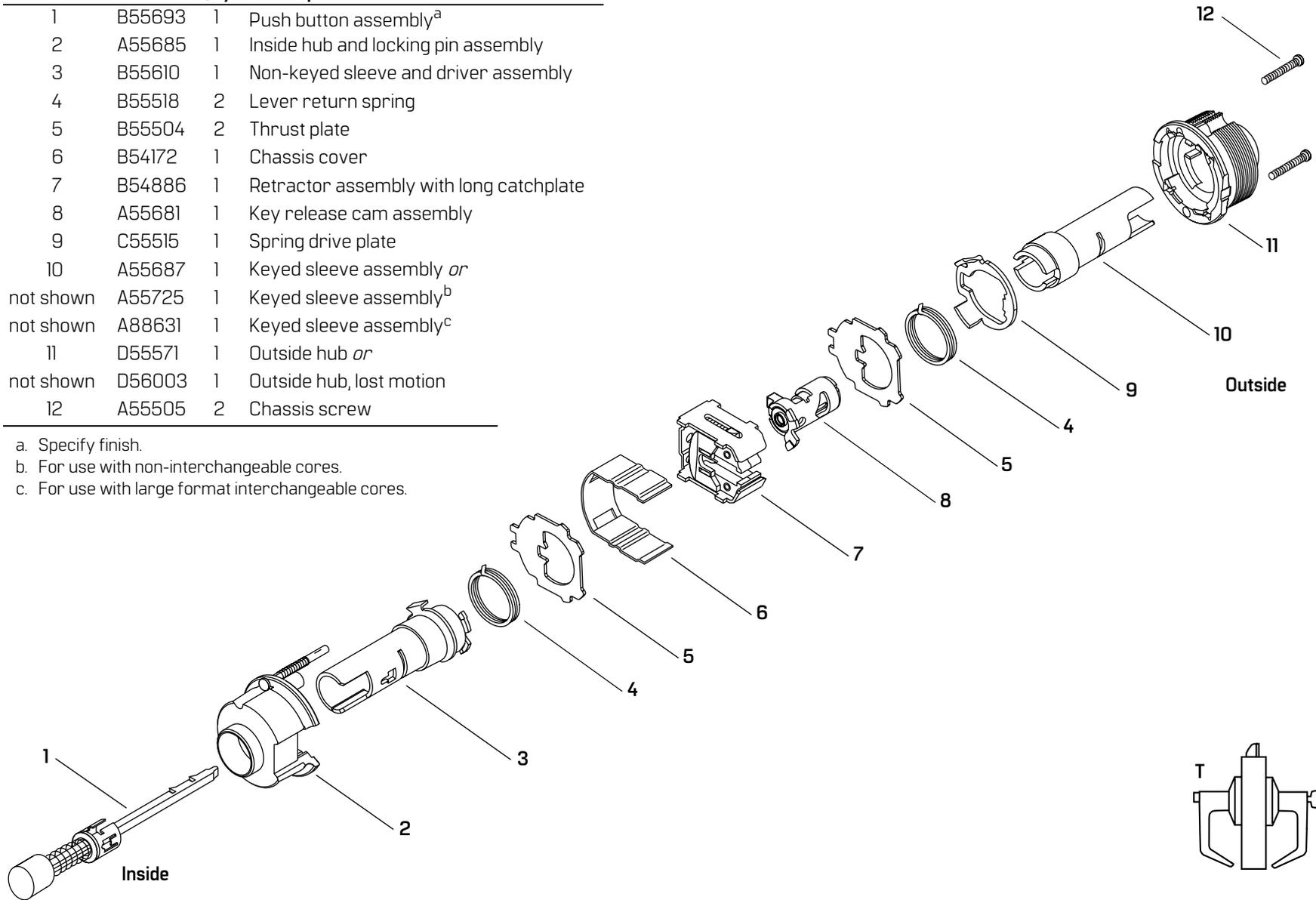
Figure 2.14 T function exploded diagram
