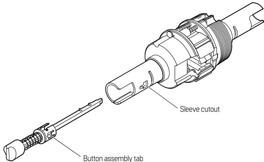
**Figure 3.11** Inserting the button assembly into the sleeve
