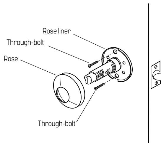
**Figure 3.7** Replacing the inside rose and rose liner
