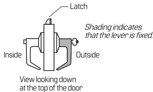
**Figure 2.1** Understanding function drawings
