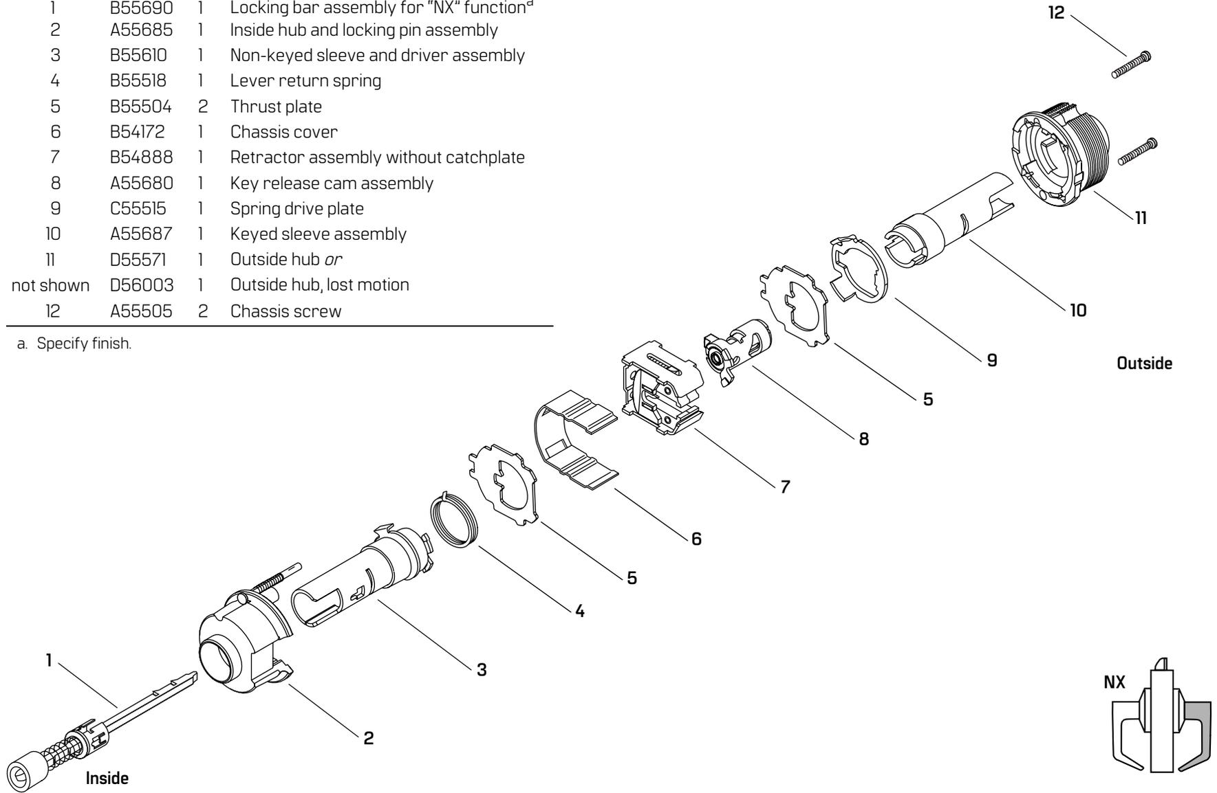
Figure 2.10 NX function exploded diagram
