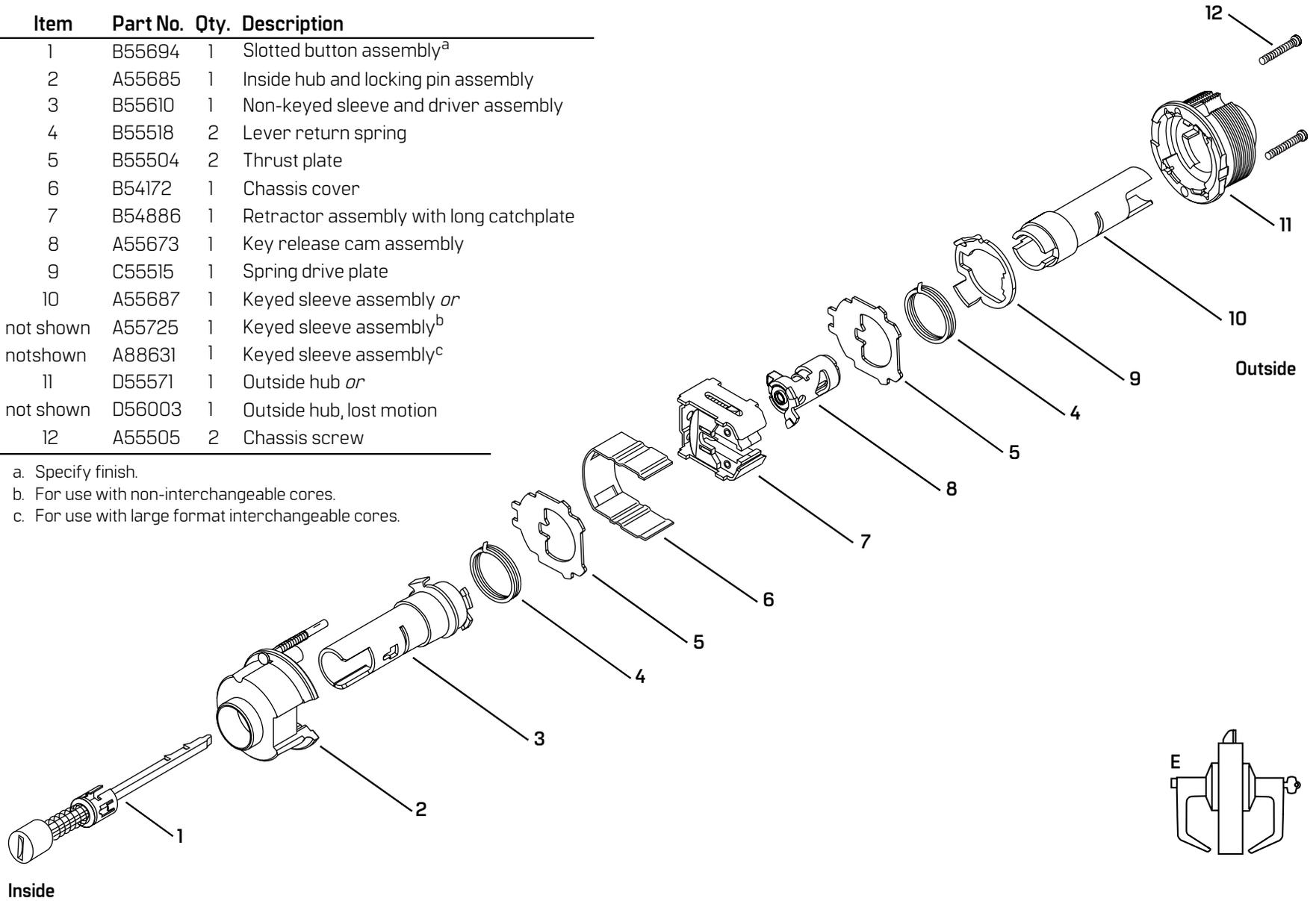
Figure 2.5 E function exploded diagram
