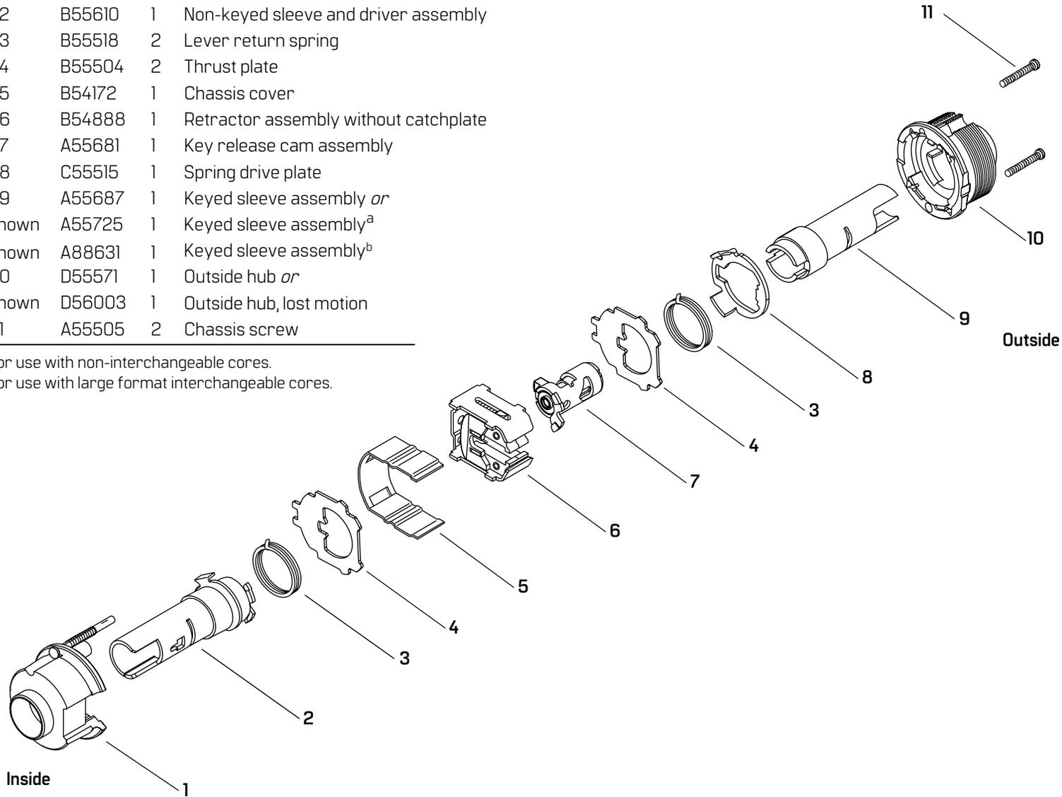
Figure 2.12 R function exploded diagram
