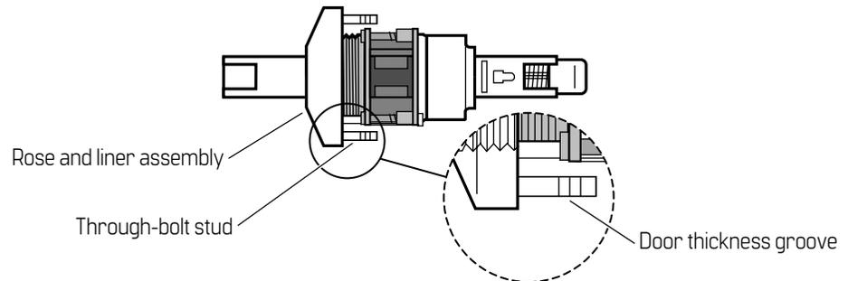
**Figure 3.9** Replacing the outside rose and liner assembly
