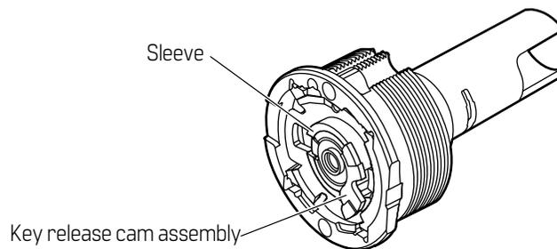
**Figure 3.24** Removing the key release cam assembly
