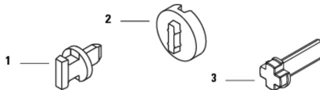
Figure 2.41 Lever components with interchangeable cores
