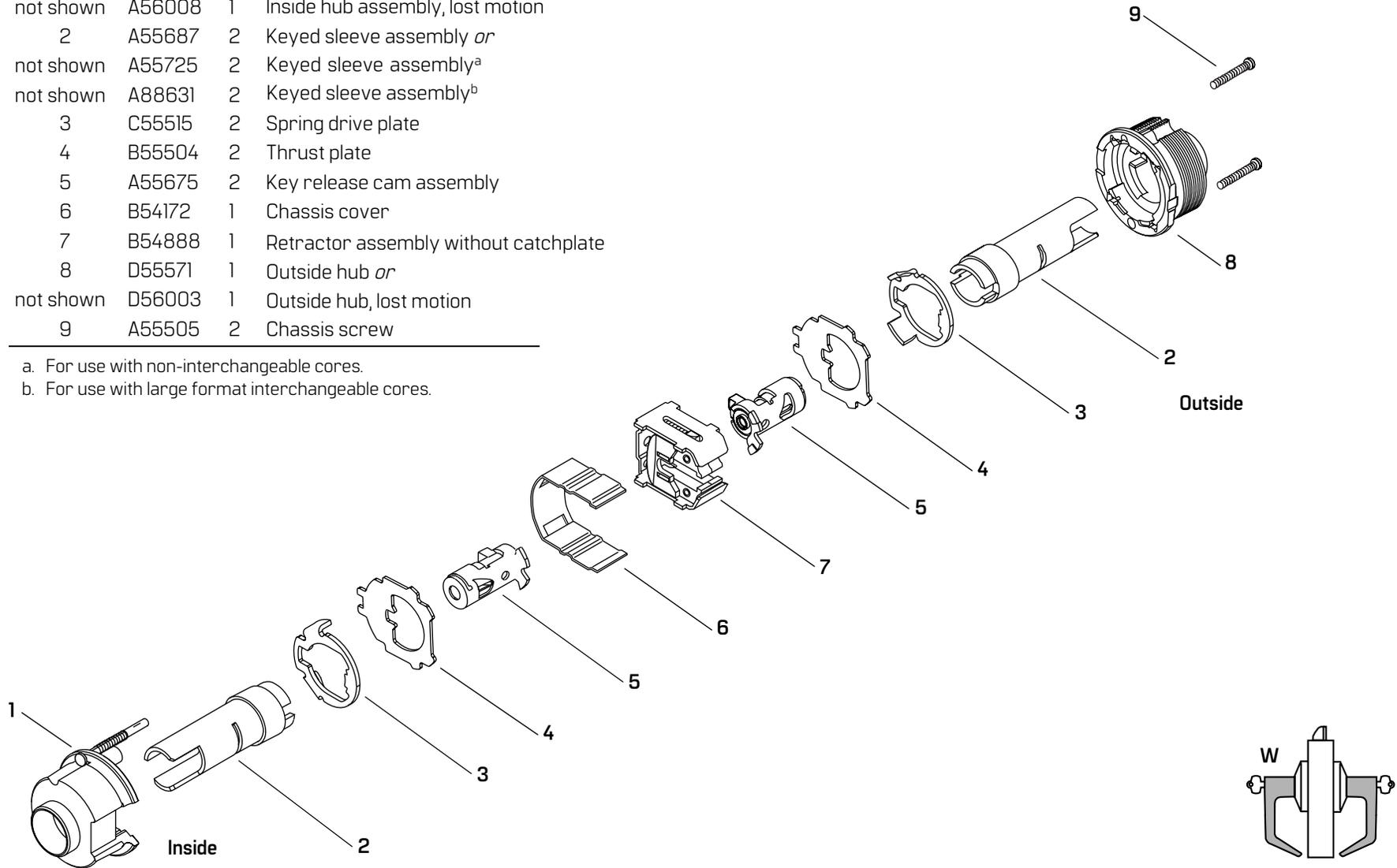
Figure 2.15 W function exploded diagram
