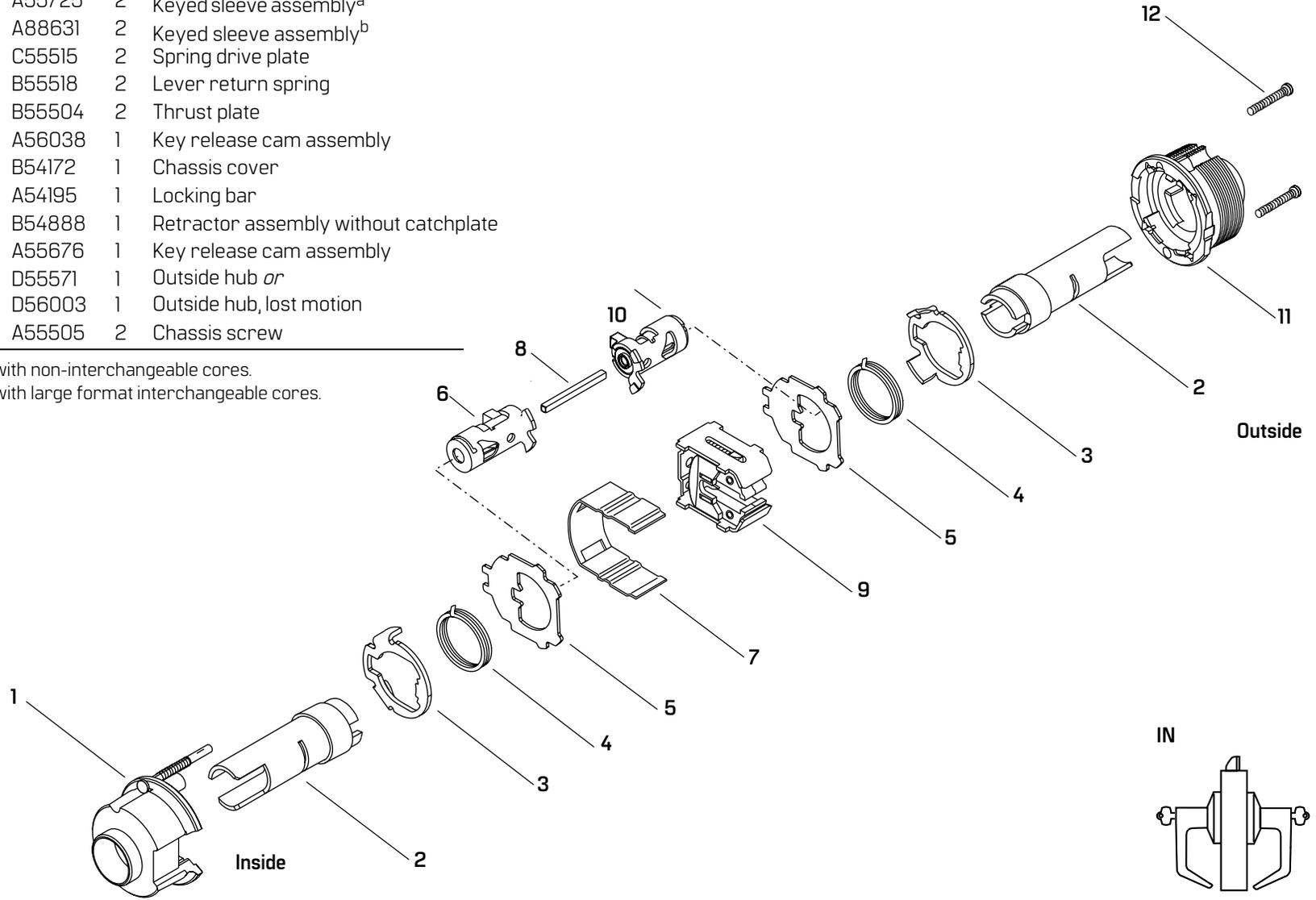
Figure 2.22 IN function exploded diagram
