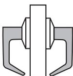
This lock is a through-bolt mounted pair of matching levers for an inactive door or a non-latching door.
