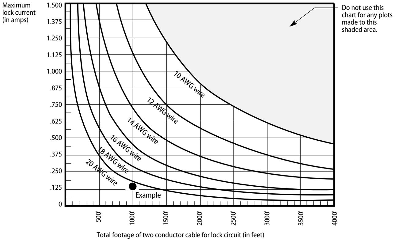
Figure 2—Minimum gauge wire chart for lock circuits
