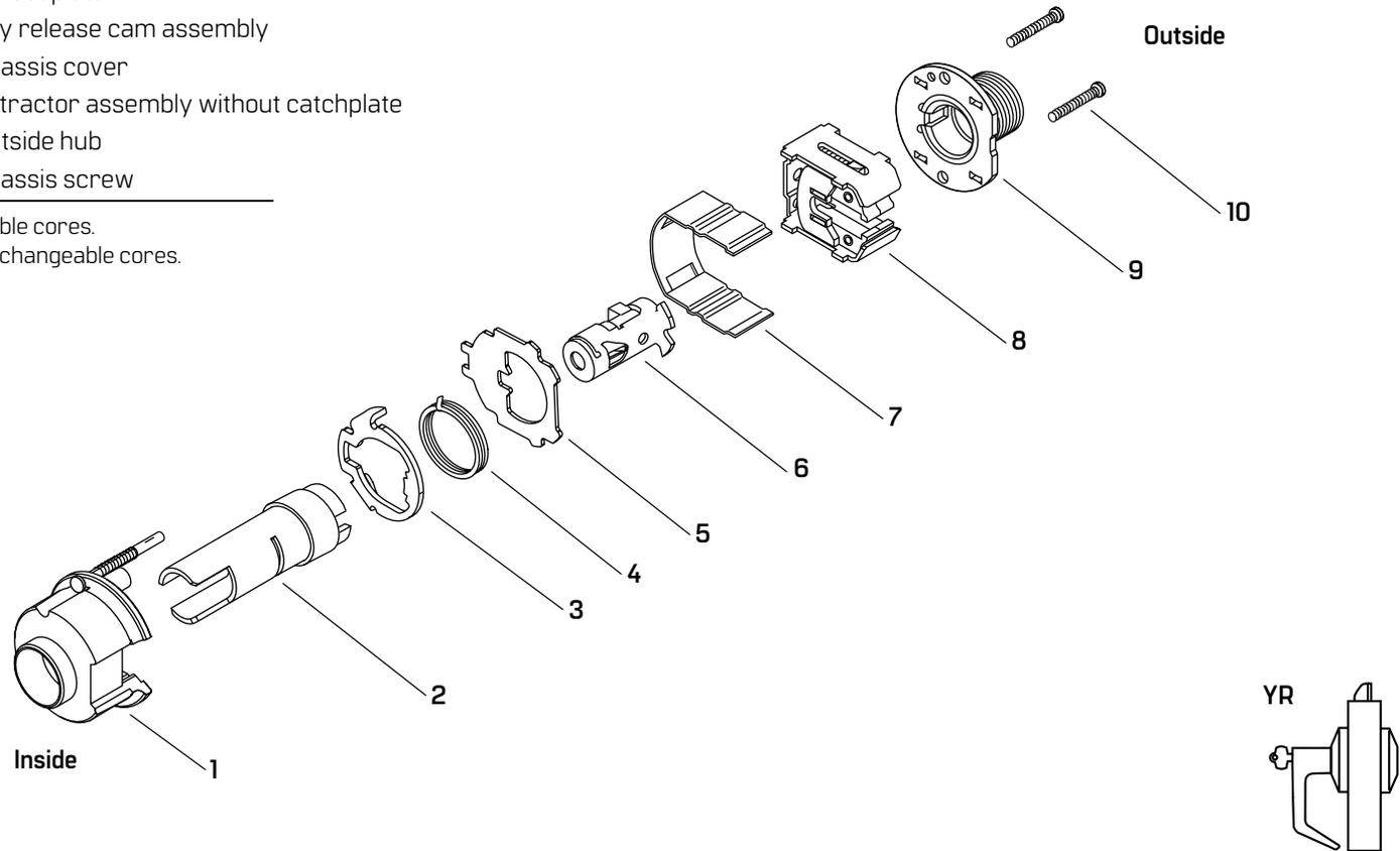
Figure 2.31 YR function exploded diagram
