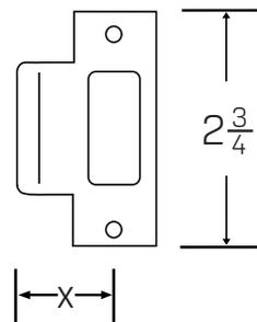
The measurement is taken from the edge of the lip to the center of the screw holes.
