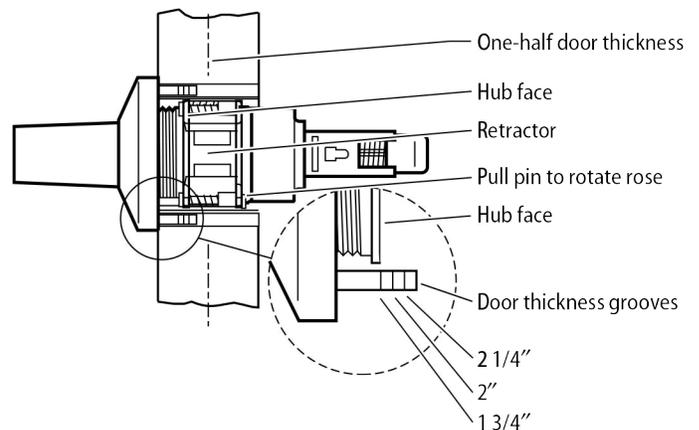
Figure 4 — Adjusting the lock chassis for door thickness
