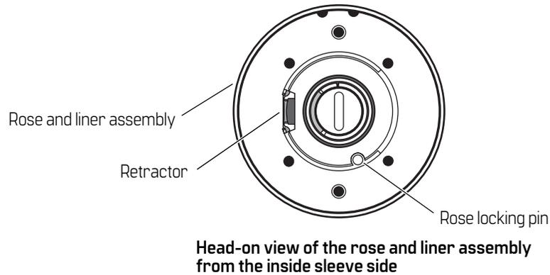
**Figure 3.8** Removing the outside rose and liner assembly
