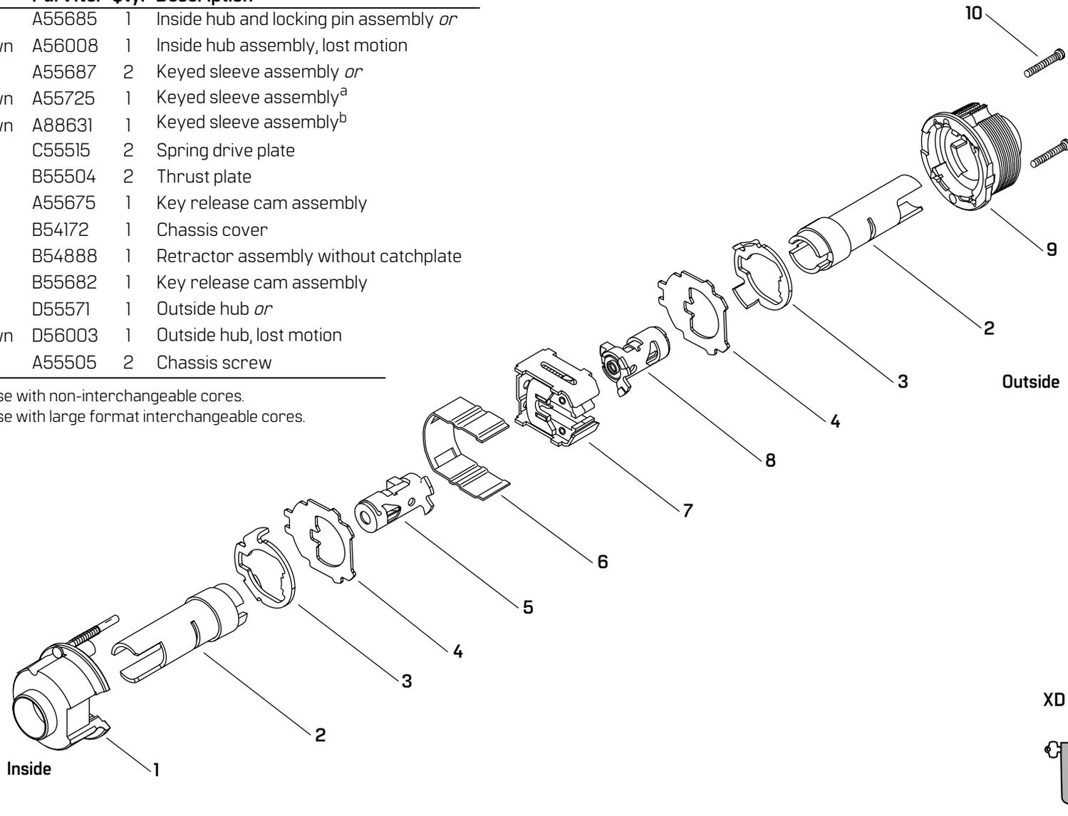
Figure 2.28 XD function exploded diagram
