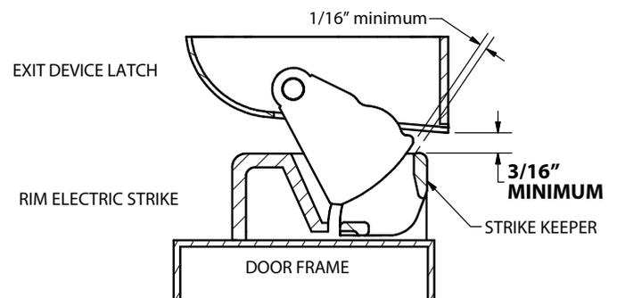
8. Tighten the two mounting screws and check operation. Adjust the horizontal position of electric strike as required.
