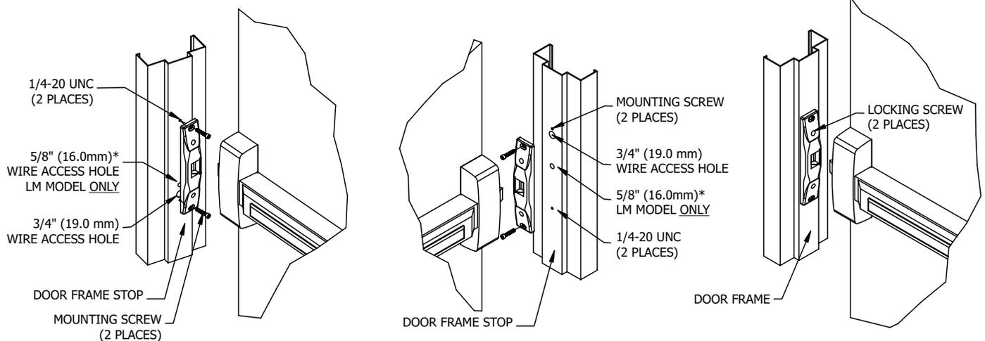
**NOTE:** Wire access hole locations are relative to the exit device orientation. **NOTE:** \*Second wire access hole required for BES-0162LM only
