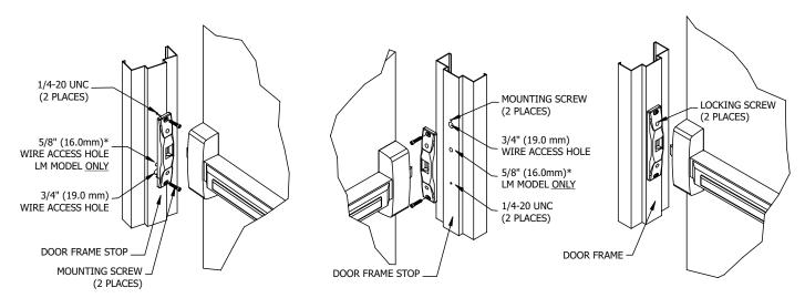
**NOTE**: Wire access hole locations are relative to the exit device orientation. **NOTE**: \*Second wire access hole required for BES-0162LM only **NOTE**: Not to scale. Specifications are subject to change without notice.
