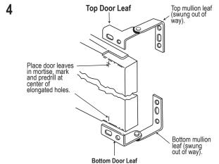
To allow for vertical adjustment and sufficient clearnace under the door, the bottom mullion leaf should be mounted at least '¼" off the floor. If carpet or other special floor coverings are used, additional clearance should be allowed equal to their thickness.
