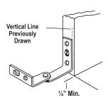
Apply bottom hinge to face of mullion using the center of the elongated hole. Be sure to line up with previously drawn vertical line
