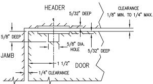
PREPARE 1" DIAMETER CUT OUT IN THE TOP OF THE DOOR AND HEADER.
