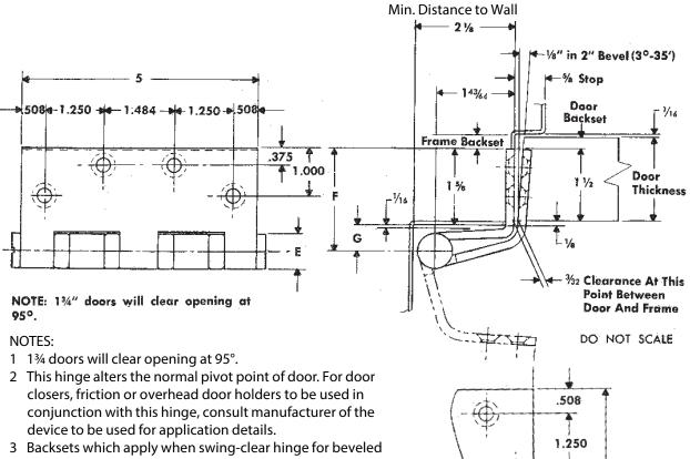
a Backsets which apply when swing-clear hinge for beveled edge hinge stile is used on door thickness indicated and when the usual 1/16 stop clearance is desired.
