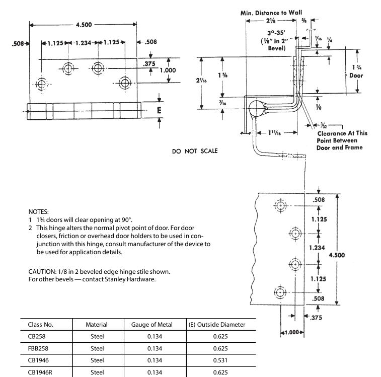
Template hinges of the hospital type conform to above screw hole location. Hospital type hinges are designated by prefix "HT" to class number.
