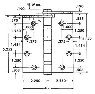
For use with door holders, closers and operators which interfere with standard door plates shown on template T50-08.
