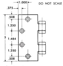
Machine Screw Size —  $\frac{1}{2} \times 12-24$  F.H. Wood Screw Size —  $\frac{1}{2} \times No.$  12 F.H.
