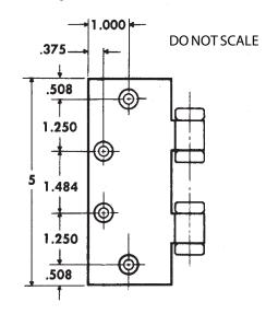
Machine Screw Size —  $\frac{1}{2} \times 12-24$  F.H. Wood Screw Size —  $\frac{1}{2} \times No. 12$  F.H.
