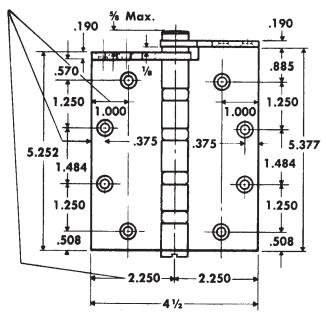
For use with door holders, closers and operators which interfere with standard door plates shown on template T50-09.
