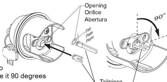
1. Insert the tailpiece in a vertical position, (perpendicular to the flat of the opening) then rotate it 90 degrees clockwise to a horizontal position.
