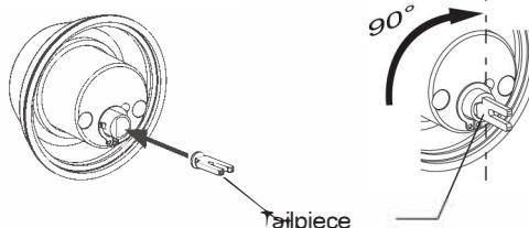
2. Insert the tailpiece horizontally, (perpendicular to the flat of the opening) then rotate it 90 degrees clockwise to a vertical position.
