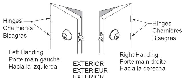
Determine door handing by facing outside of door. Door hinges will be on the left for **left handing**; door hinges will be on the right for **right handing**.
