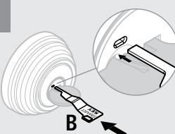
Insert SmartKey tool (B) fully and firmly into the hole. You may feel the tool click inside the lock.
