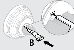
Insert the SmartKey tool (B) fully and firmly into the hole. You may feel the tool click inside the lock.
