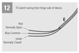
TDS Switch wiring from hinge side of device. (D.P.D.T. Option)
