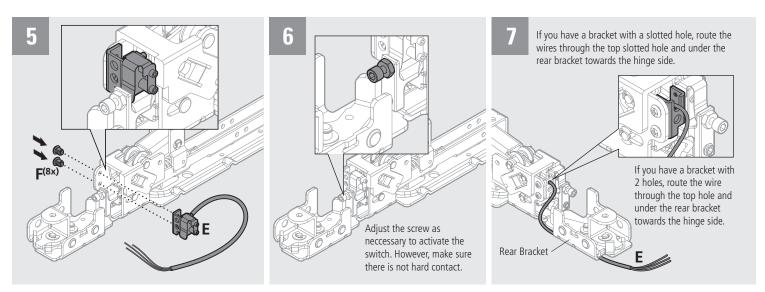
Do not pinch wires and ensure they are not coming into contact with any moving parts.
