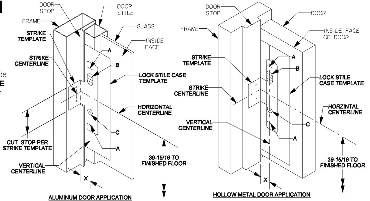
4. Tape Lock Stile Case Template (and Trim Template if Trim specified) to the door so that the centerlines on the Template line up with centerlines on the door. Mark centers and drill the required holes as indicated on the templates.
