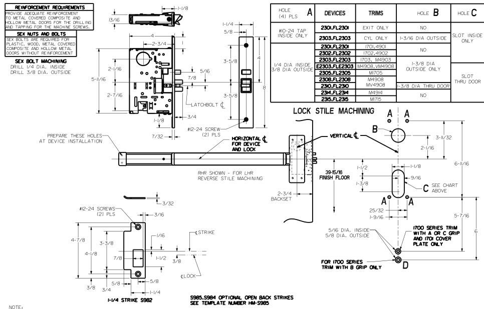
"LETTER" AT END OF TRIM MODEL NO. DESIGNATES LEVER OR GRIP STYLE. EXCEPT AS NOTED, LEVER OR GRIP STYLE HAS NO EFFECT ON STILE MACHINING.
