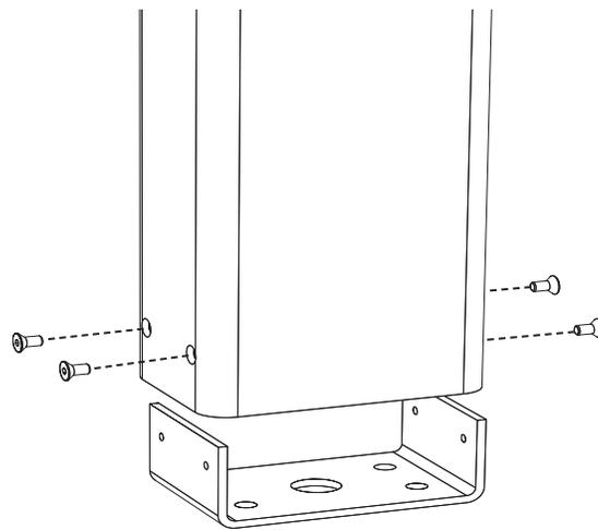
1. Align post to mounting bracket and attach post to mounting bracket with four post mounting screws.
