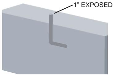
2. Insert anchors into curing concrete. Leave at least 1 inch exposed.
