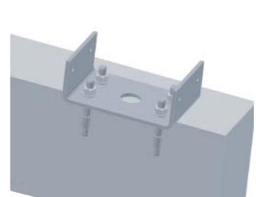
3. Install and tighten nuts to secure mounting bracket.
