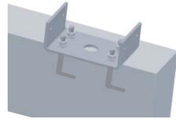
3. Once concrete has cured attach anchor and tighten nuts onto mounting bracket.
