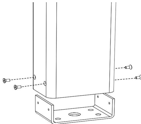
1. Align post to mounting bracket and attach post to mounting bracket with four post mounting screws.
