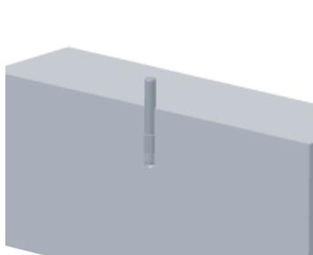
2. Hammer in and set anchor in four hole locations.
