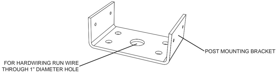
1. The Bollard is designed to house a pushplate used to activate a door by either a remote controlled transmitter or hardwired directly to the door control. If the door is hardwired, pass the wire through the 1 inch diameter hole in the mounting bracket.
