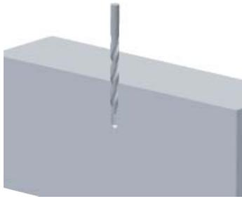
1. Mark and drill 3/8" diameter hole in four locations.
