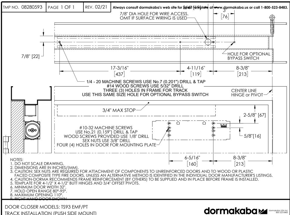
TRACK INSTALLATION (PUSH SIDE MOUNT) WITHOUT SMOKE DETECTOR
