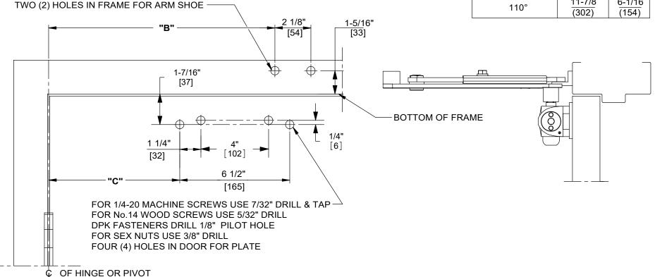
DOOR CLOSER MODELS: 7400 IS, ISH REGULAR INSTALLATION (PULL SIDE MOUNT) DEAD STOP ARM WITH PLATES BP74, BP86, BP86FC
