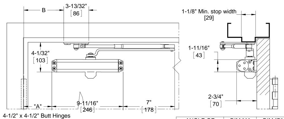
Minimum door rail for mounting closer 4-3/8" (5/8" stop shown). Minimum door rail to the bottom of slim plastic cover 4-1/2".
