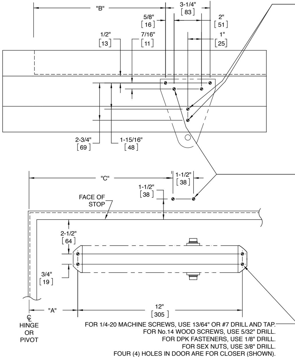
\*IMPORTANT CHOOSE APPROPRIATE FIFTH HOLE LOCATION FOR SPACER BLOCK, IN ACCORDANCE WITH FRAME WIDTH. ONE (1) HOLE IN FRAME FOR STANDARD BLOCK. PREPARE HOLE THE SAME AS SOFFIT PLATE HOLES.
