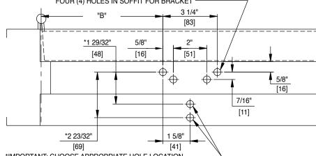
\*IMPORTANT: CHOOSE APPROPRIATE HOLE LOCATION FOR SPACER BLOCK, IN ACCORDANCE WITH FRAME WIDTH.
