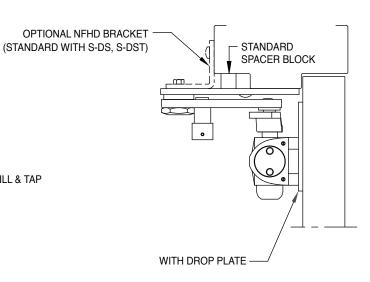
FOR SEX NUTS USE 3/8" DRILL FOUR (4) HOLES IN DOOR FOR PLATE
