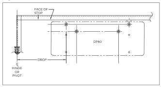
Fig. 7 Plate and closer attachment
