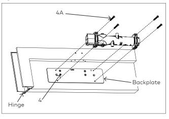
Fig. 9 Plate and closer attachment
