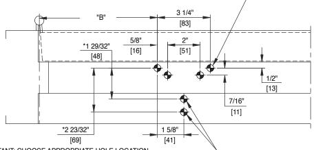
\*IMPORTANT: CHOOSE APPROPRIATE HOLE LOCATION ------FOR SPACER BLOCK, IN ACCORDANCE WITH FRAME WIDTH.
