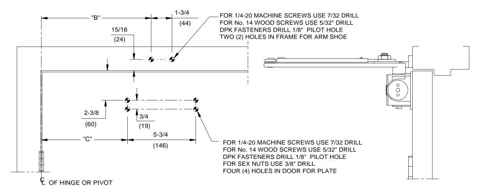
DOOR CLOSER MODELS: 8916, 8956 FH REGULAR INSTALLATION (PULL SIDE MOUNT) WITH PLATE BP89
