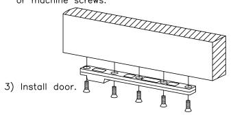
With door parallel to frame, place bottom arm onto spindle. Rotate door approximately 90°. Align bearing with pivot pin. Engage pivot pin by turning adjustment screw clockwise. Check to make sure pivot pin is fully engaged in door portion of pivot.
