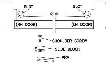
Place arm over spindle. Seat arm properly on spindle by tapping with hammer. Install cover washer and screw.
