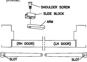
5 Slide arm assembly into track and install track into door.
