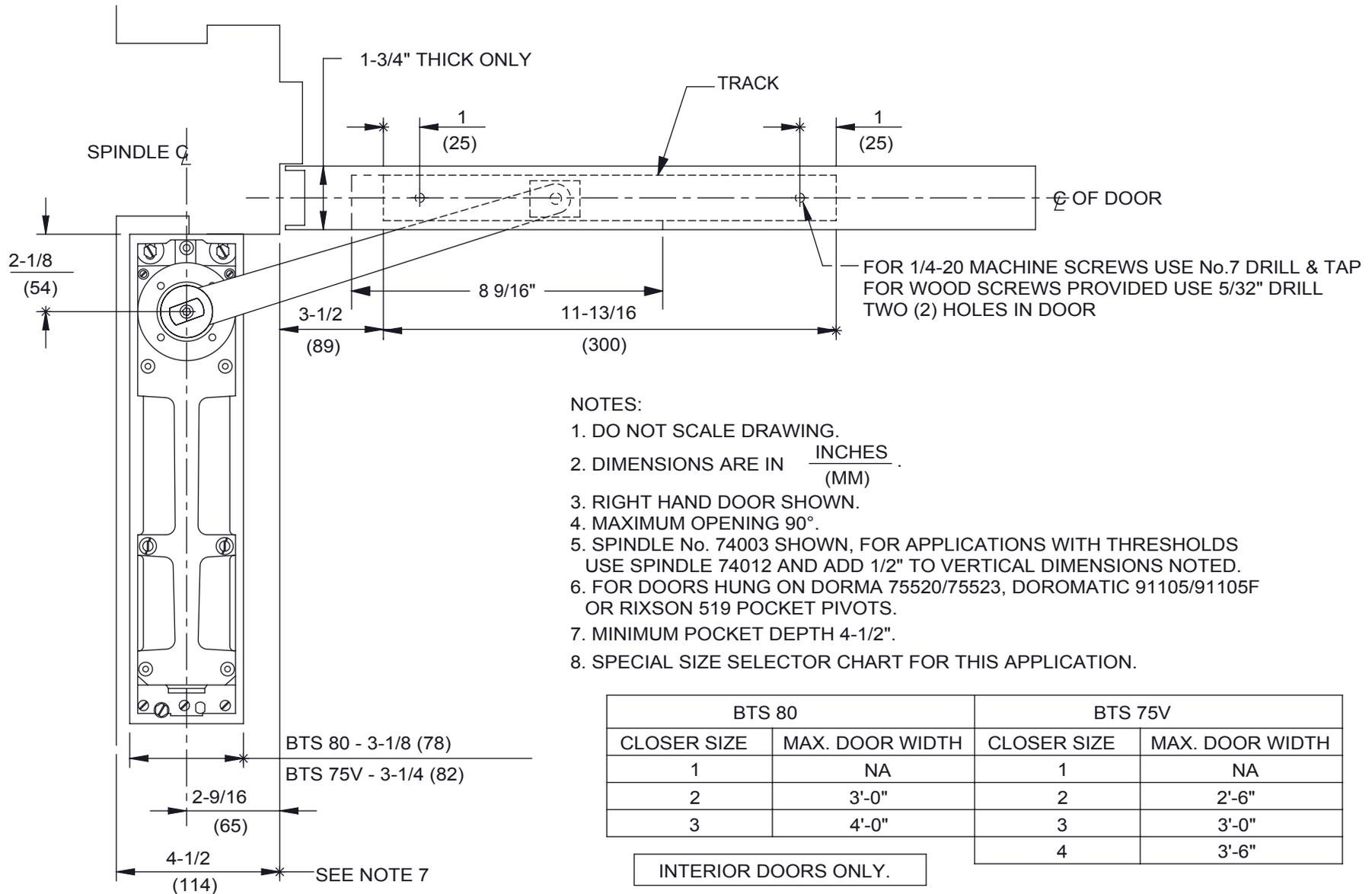
FLOOR CLOSER MODEL: BTS 75V/P, 80/P WITH 7451N SLIDE ARM ASSEMBLY
