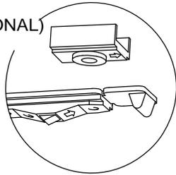
NOTE: ARROWS ON HOLD OPEN AND SLIDE SHOE, MUST POINT AWAY FROM HINGE WHEN INSTALLING IN TRACK.
