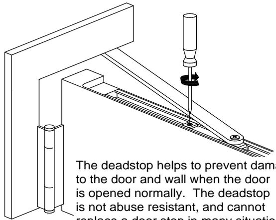
The deadstop helps to prevent damage to the door and wall when the door is opened normally. The deadstop is not abuse resistant, and cannot replace a door stop in many situations. Deadstop is adjustable between 80° and 120° maximum.
