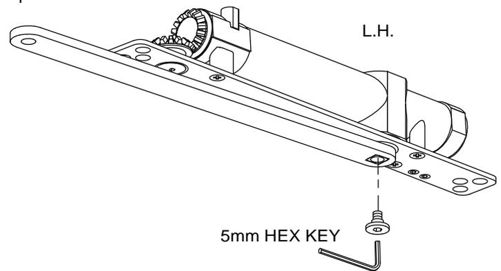
4 Close valve by turning completely clockwise. Rotate arm 45° and attach closer to frame.
