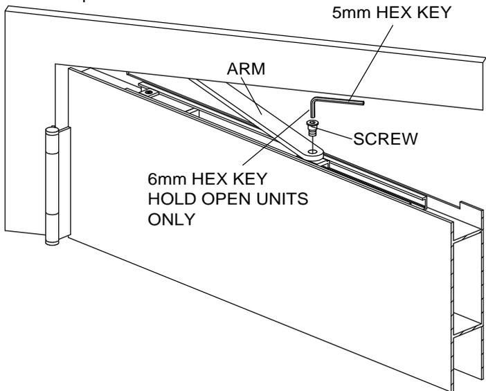
7 Open door to desired opening between 80° and 120°. Tighten deadstop block.
