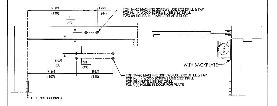
DOOR CLOSER MODELS: 8916 AR STA REGULAR INSTALLATION (PULL SIDE MOUNT) WITH PLATE BP89
