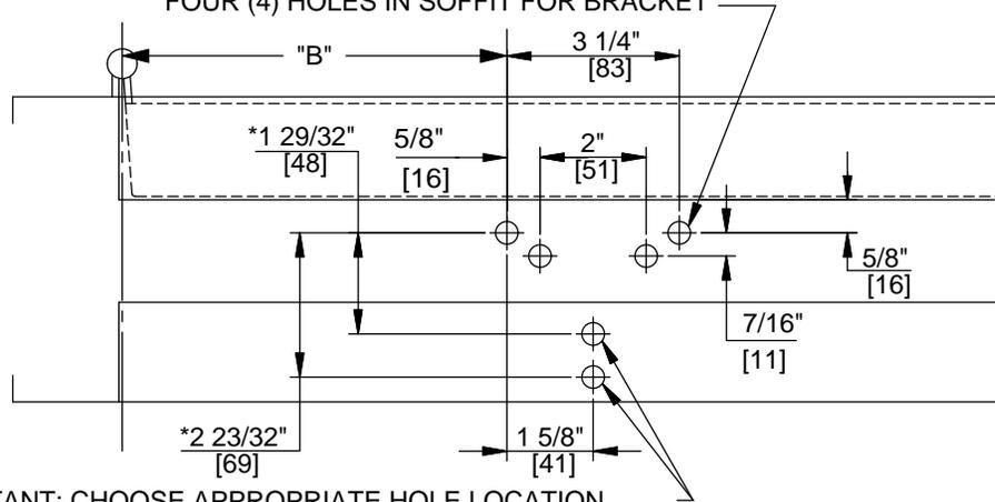
\*IMPORTANT: CHOOSE APPROPRIATE HOLE LOCATION FOR SPACER BLOCK, IN ACCORDANCE WITH FRAME WIDTH. ONE (1) HOLE IN FRAME FOR SPACER BLOCK.
