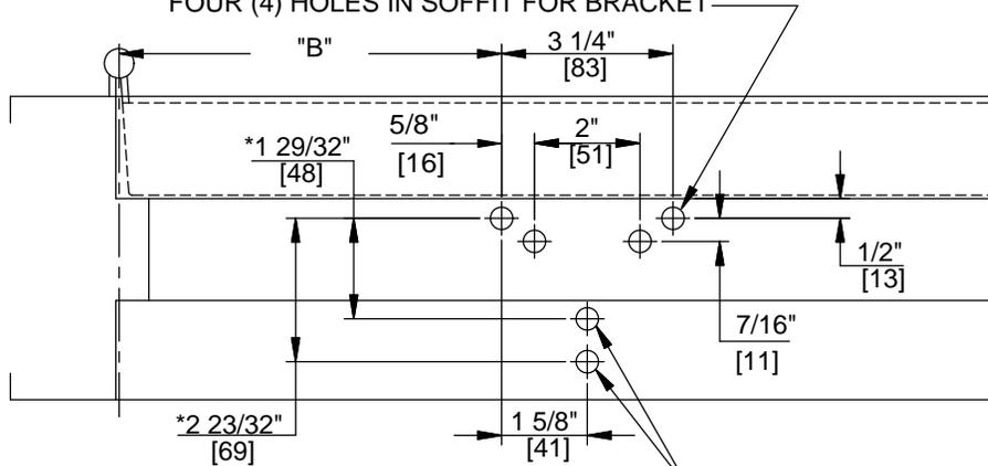
\*IMPORTANT: CHOOSE APPROPRIATE HOLE LOCATION FOR SPACER BLOCK, IN ACCORDANCE WITH FRAME WIDTH. ONE (1) HOLE IN FRAME FOR SPACER BLOCK.
