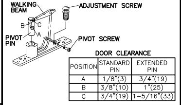
Center closer in cement case. Tighten fastening screws.
