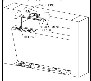
Adjust bottom door clearances. (If necessary)
