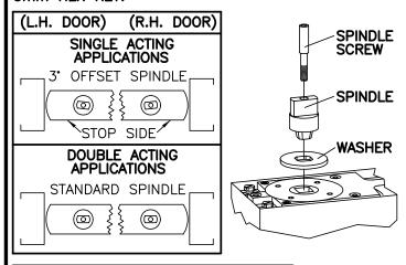
adjust projection of pivot pin, if required. Pivot pin projection allows 1/8" clearance as shipped from the factory. To change projection of pivot pin or to install
