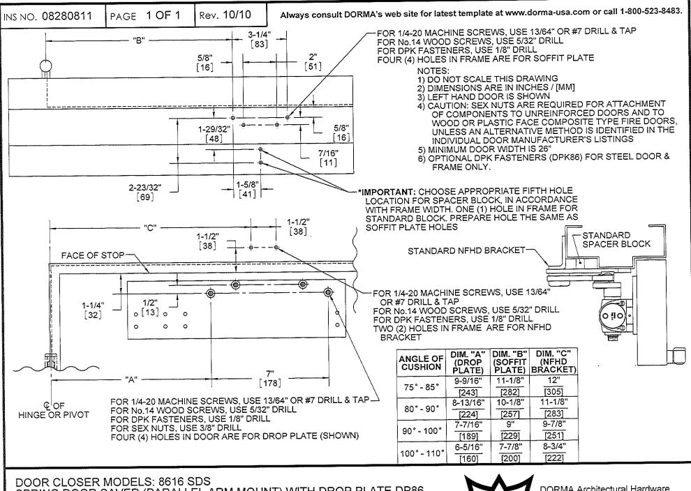
DOOR CLOSER MODELS: 8616 SDS SPRING DOOR SAVER (PARALLEL ARM MOUNT) WITH DROP PLATE DP86 FOR USE WITH STANDARD SPACER BLOCK FOR USE WITH STANDARD NFHD BRACKET
