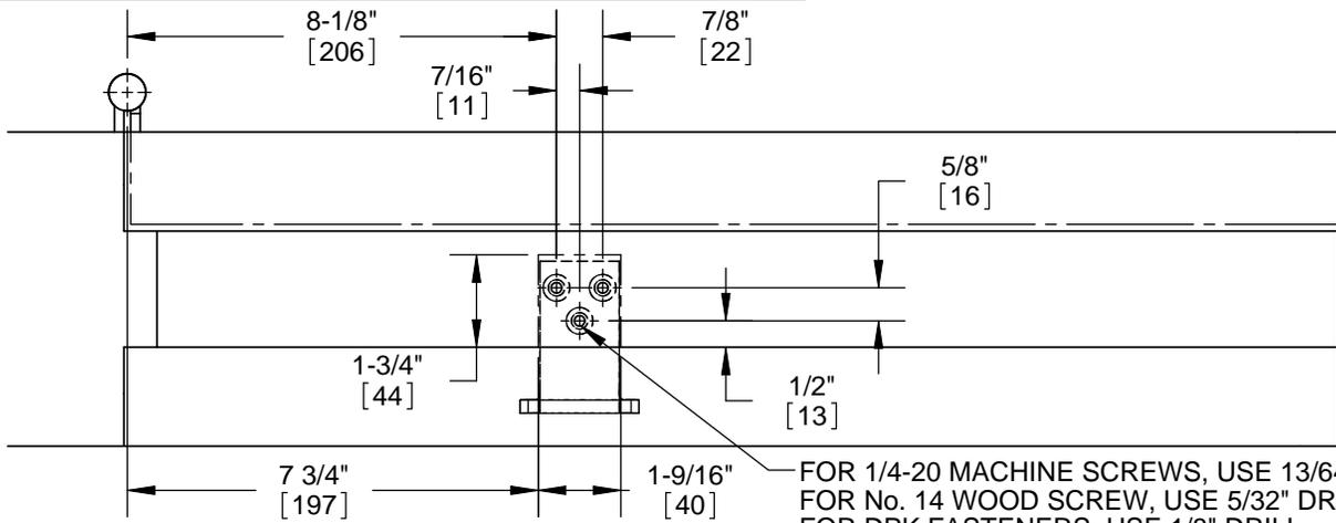
FOR 1/4-20 MACHINE SCREWS, USE 13/64" OR #7 DRILL & TAP
