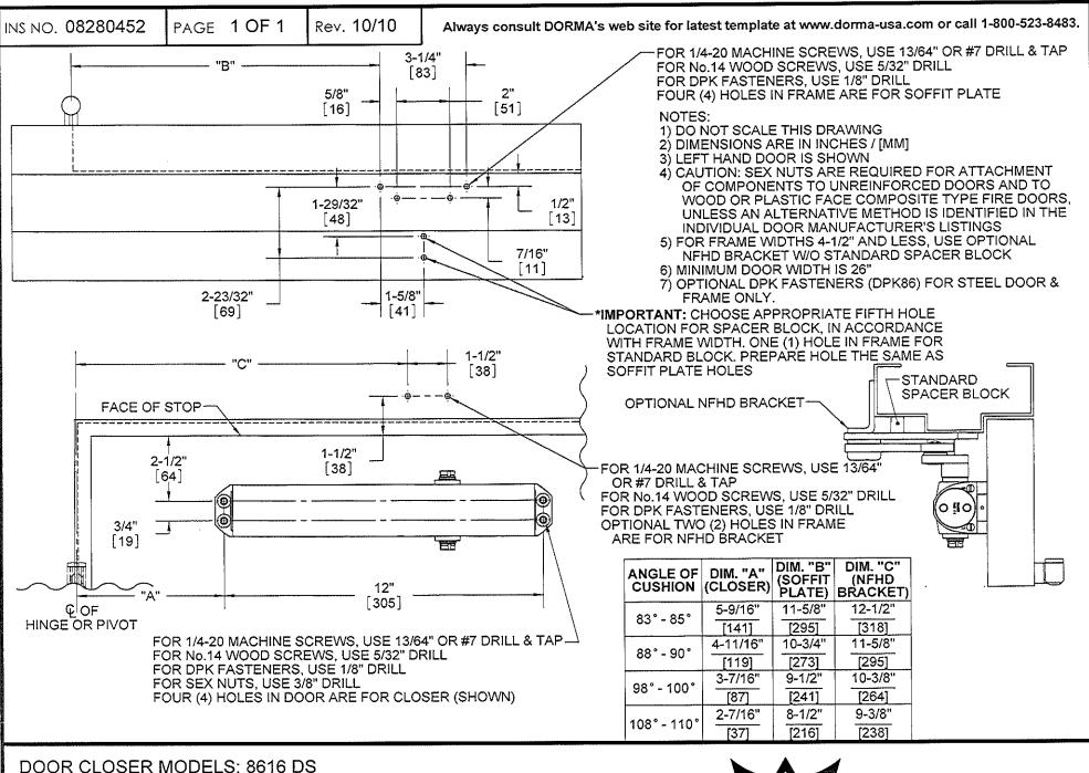
DOOR CLOSER MODELS: 8616 DS DOOR SAVER (PARALLEL ARM MOUNT) FOR USE WITH STANDARD SPACER BLOCK FOR USE WITH OPTIONAL NFHD BRACKET
