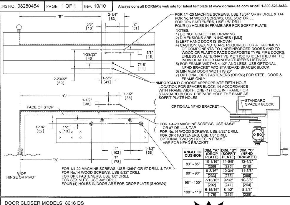
DOOR CLOSER MODELS: 8616 DS DOOR SAVER (PARALLEL ARM MOUNT) WITH DROP PLATE DP86 FOR USE WITH STANDARD SPACER BLOCK FOR USE WITH OPTIONAL NFHD BRACKET
