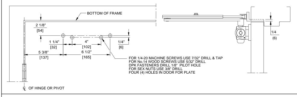
DOOR CLOSER MODELS: 8616 AF x MJ REGULAR INSTALLATION (PULL SIDE MOUNT) WITH PLATES BP86, BP86FC
