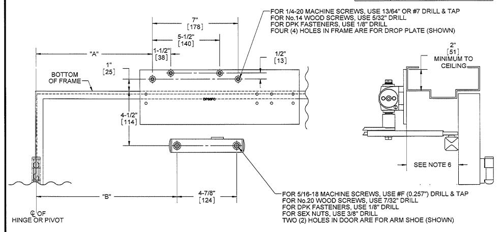
DOOR CLOSER MODELS: 8616 SISJ TOB JAMB INSTALLATION (PUSH SIDE MOUNT) WITH BACK PLATE DP86 SPRING INTEGRA CUSHION ARM
