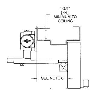
DOOR CLOSER MODELS: 8916 & 8956 SISJ TOP JAMB INSTALLATION (PUSH SIDE MOUNT) WITH DROP PLATE BP89 SPRING INTEGRA CUSHION ARM
