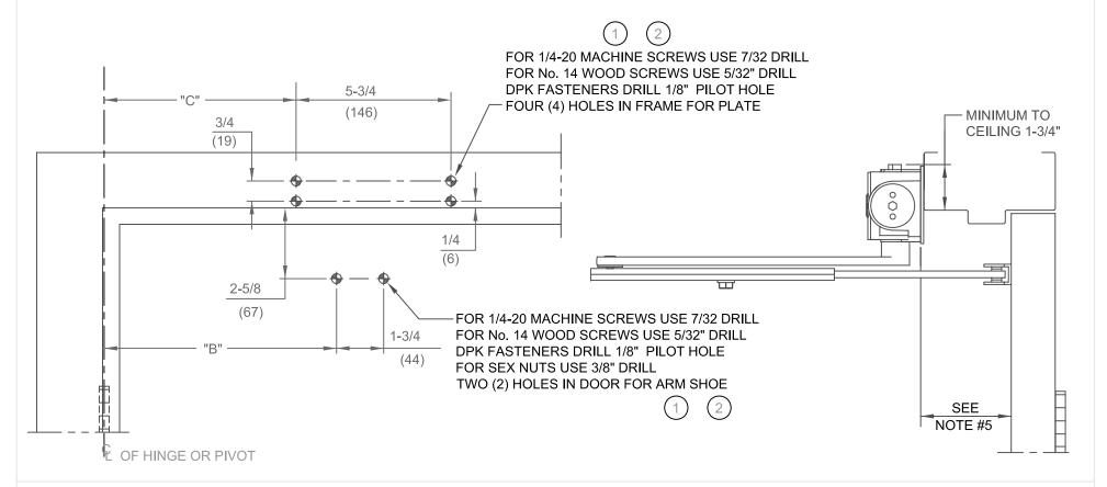
DOOR CLOSER MODELS: 8916, 8956 AF89J, PH, PHP TOP JAMB INSTALLATION (PUSH SIDE MOUNT) WITH PLATE BP89 DROP
