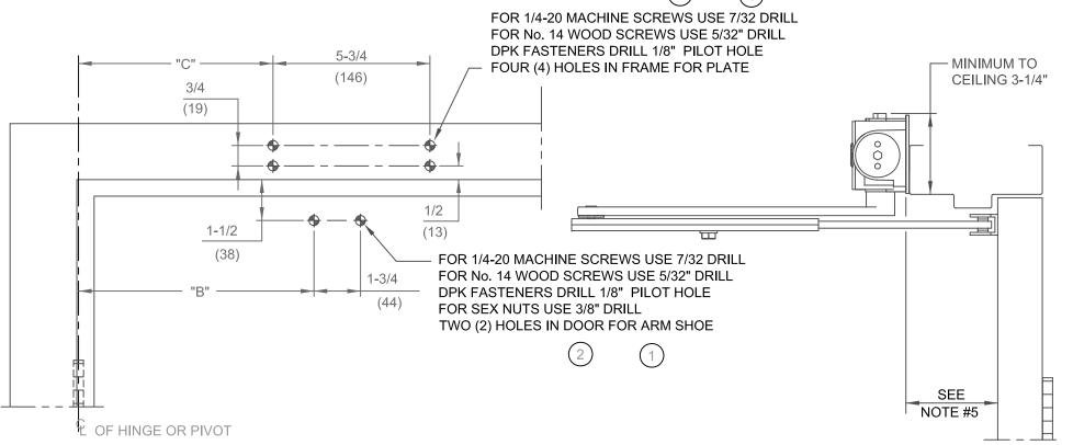
DOOR CLOSER MODELS: 8916, 8956 AF89J, PH, PHP TOP JAMB INSTALLATION (PUSH SIDE MOUNT) WITHPLATE BP89
